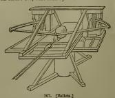
sinews, with a trigger to set it free, and contrived either to impel darts by its stroke, or to throw stones from a kind of spoon formed towards the summit of the spring.
